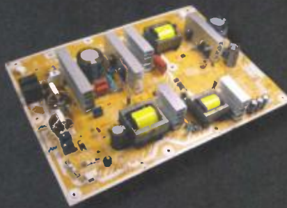
Plazma modul zdroj NOAE5JK00005 / P BOARD ASSY (SMPS) NOAE5JK00005, plazma TV Panasonic
